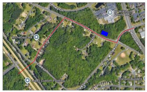
Red lines indicate the new Main installation on the aforementioned affected streets. The blue rectangle indicates the proposed Distribution Regulator location.
